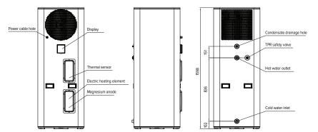
EE-HWS-A1-220E(-1) (The electric heating element is not included in EE-HWS-A1-220)
