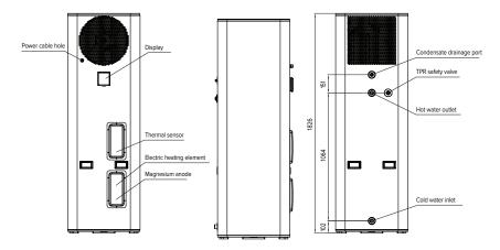
EE-HWS-A1-270E(-1) (The electric heating element is not included in EE-HWS-A1-270)
