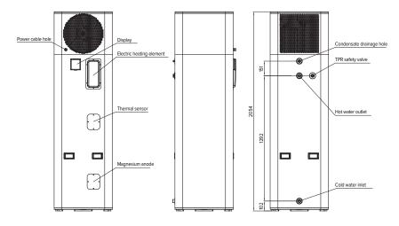
EE-HWS-A1-320E(-1) (The electric heating element is not included in EE-HWS-A1-320)
